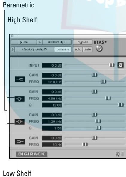
Figure 3-3: The 4-band EQ in Pro Tools lets you apply four EQ filters to a track.
